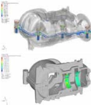
Drill hammer gear housing structural analysis for assembly and operating loads using OptiStruct®.
