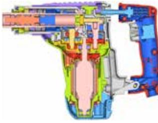
Detailed cutaway view of DeWalt's hammer drill finite-element model developed using HyperMesh®.
