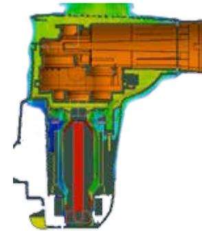
Drill hammer airflow simulation using AcuSolve®.
