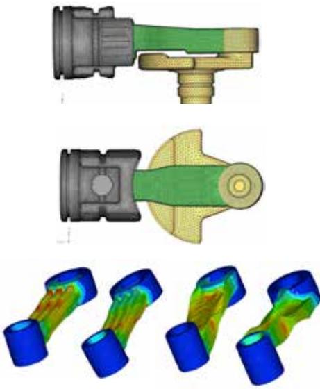
DeWalt engineers apply co-simulation to improve the performance of products using Altair's OptiStruct® topology optimization and MotionSolve® multi-body dynamics analysis technologies. Redesigning this connecting rod using co-simulation resulted in a 25% reduction in maximum stress level and a lighter weight product.
