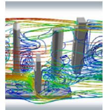
Virtual wind tunnel testing produces accurate modeling of wind pressures and enables designers to explore and evolve concepts based on CFD insights
