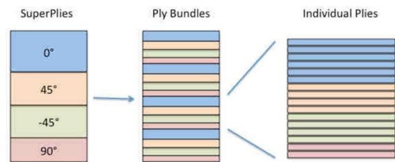
Fig 6: Schematic of "super ply", ply bundles and individual plies
