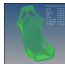
Fig 3: Elements violating thresholds
