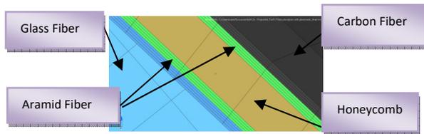
Fig 4: Composition of the laminate according to material
