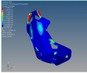
Fig 7: Element thicknesses before ply bundle optimization
