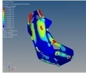
Fig 8: Element thicknesses after ply bundle optimization (discrete sizing optimization)
