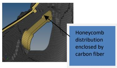
Fig 9: Position of Honeycomb in the structure
