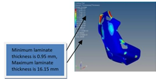
Fig 5: Element Thicknesses
