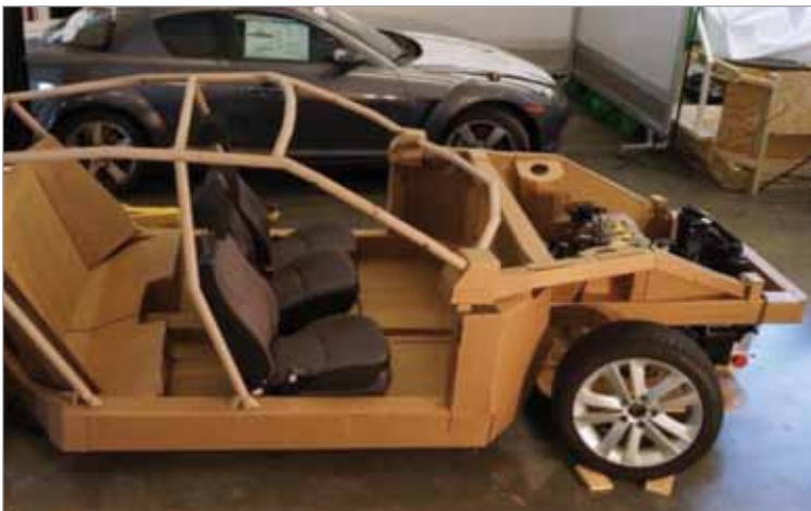
Vehicle FMT Card Board Mock Up with Front Seating Configuration
