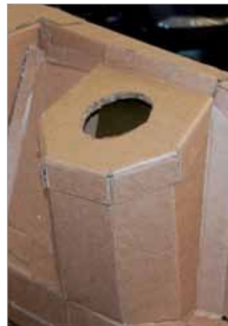
Vehicle FMT CardBoard Mock-Up for Shock Tower
