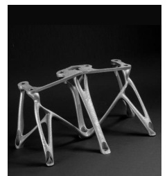
Final part after Support Removal
