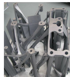
Build Platform after Manufacturing
