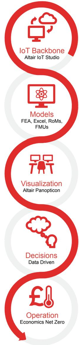
The digital twin uses a cloud native IoT platform and visualization leveraging existing FEA models to drive critical decisions that improve plant operation and maintenance.
