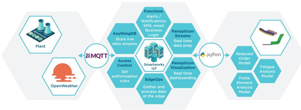
Altair IoT Studio leverages a web-of-things concept to connect plant operational data to physics-models and provides a visualization layer to get all the insights from the digital twin in real-time
