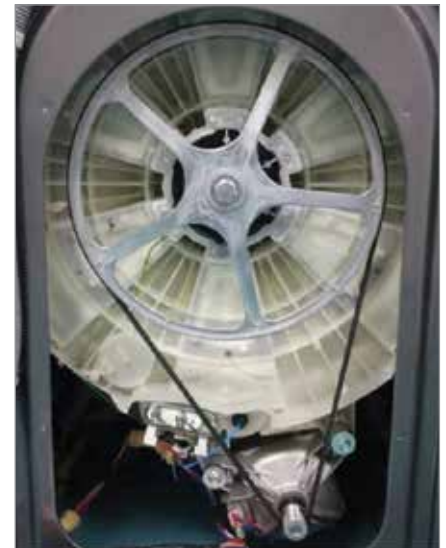
The original aluminum belt pulley installed on a washing machine
