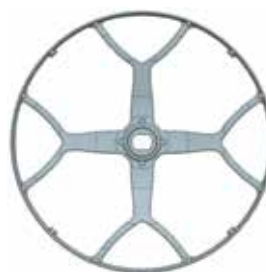
Optimized CAD model of four-spoke aluminum-based belt pulley
