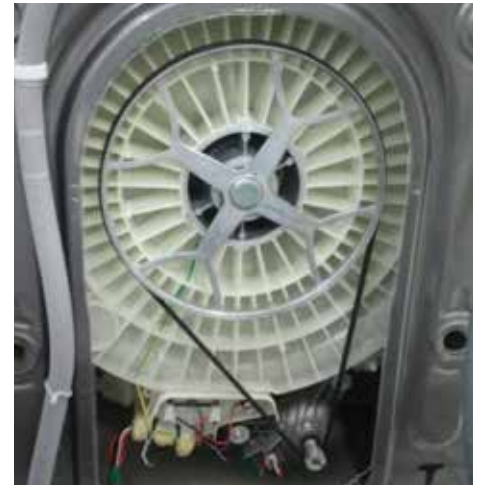
The optimized four-spoke aluminum belt pulley runs in mass production
