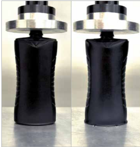
Instron Top Load Test showing deformation of actual 22g bottle
