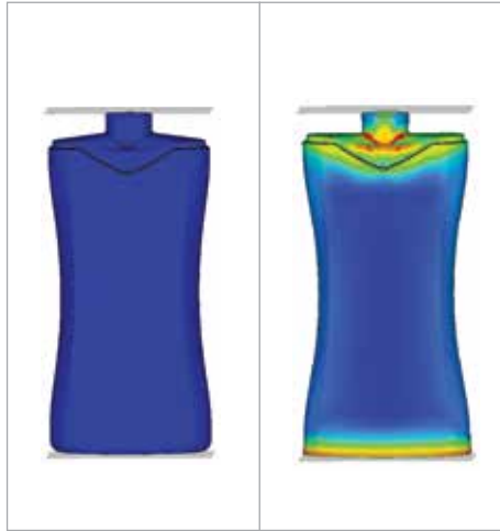
Top Load Simulation showing wall thickness and deformation of 22g bottle
