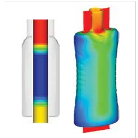
Blow mold Simulation mimicking wall thickness on actual 22g bottle
