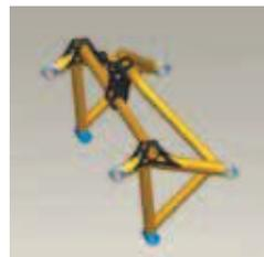
For a new suspension arm assembly, designers at Polaris started from the existing welded-tube design
