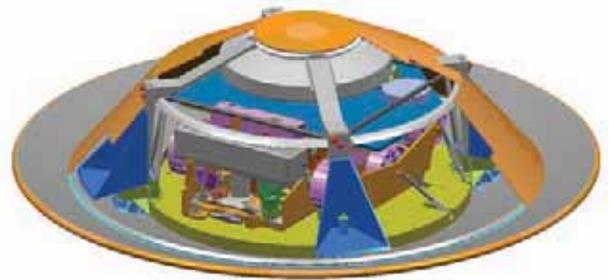
**ExoMars Descent Module with stowed Rover and packed airbag**
