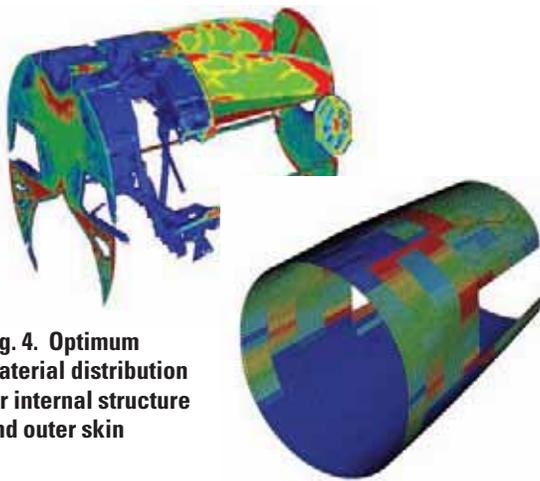
**Fig. 4. Optimum material distribution for internal structure and outer skin**
