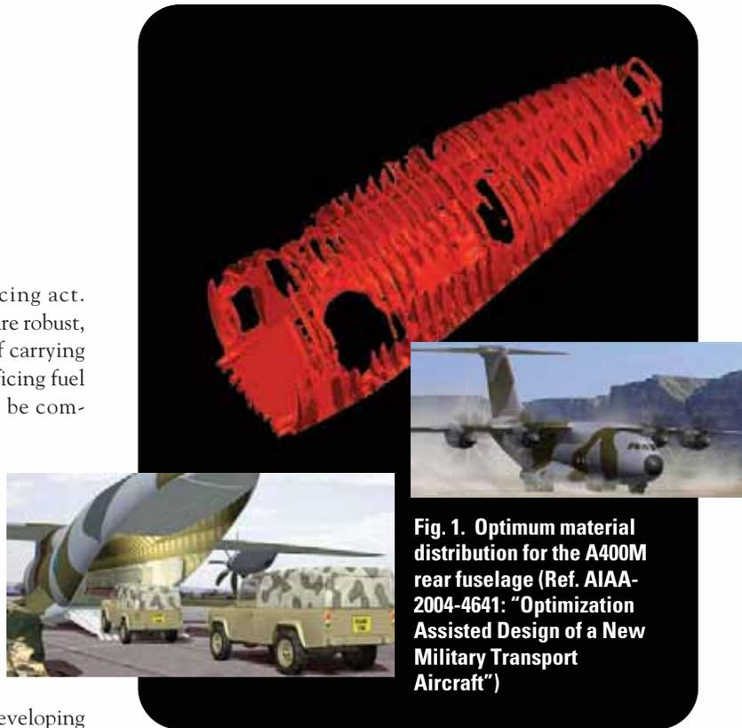
**Fig. 1. Optimum material distribution for the A400M rear fuselage (Ref. AIAA-2004-4641: “Optimization Assisted Design of a New Military Transport Aircraft”)**
