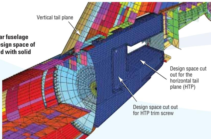
**Fig. 3. A350 rear fuselage half-model: Design space of section 19 filled with solid elements**
