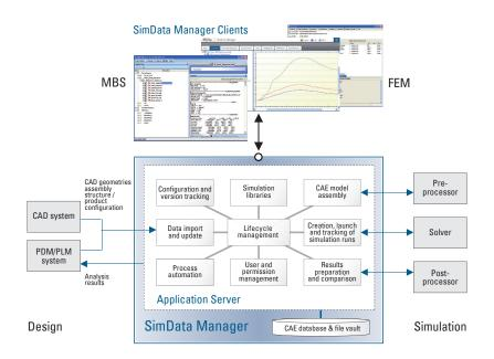
With SimData Manager, you can trace CAD geometries back from the simulation models (FE assemblies, etc.) and analyses – there is no need to manually maintain dependencies. You will always know what geometries were used to build the simulation models and obtain the analysis results. By applying this knowledge to new geometries, you can reduce the time and effort needed to collect and prepare data.
