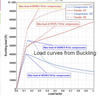
With 10 g reduction in mass, the second shell design exceeds the buckling loads. This shows the significance of running a free size that redistributes the material efficiently to meet the targets with reduced mass. Upon further investigation it is observed that the max stress occurs at a transition and can be addressed by smoothing the features.
