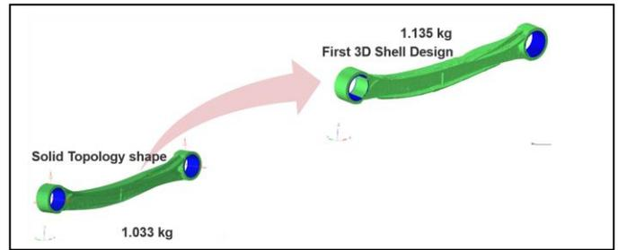
The following table shows the design performance of all load cases after converting the topology geometry to shell mesh model without CAD intervention. Buckling and Durability (stress) being the driving load cases for optimization, the first shell design shows that it is marginally underperforming in Buckling and Durability.
